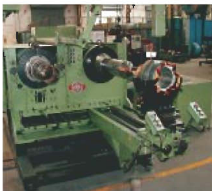
Automatic Winding Machine, STATOMAT - Germany
